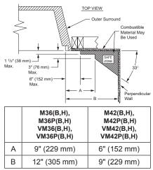
Figure 6 - Side Clearances - Top View (Cross Section)
